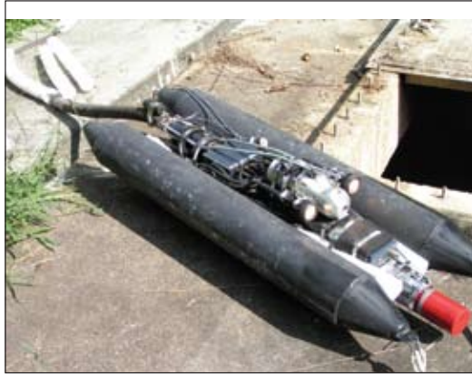
The inspection contractor used a floating transport with closed-circuit television and sonar sensor technologies to inspect about 21,000 ft (6400 m) of the Shades Valley Transfer line. Track-mounted inspection equipment couldn't fit through the line's access structures.
